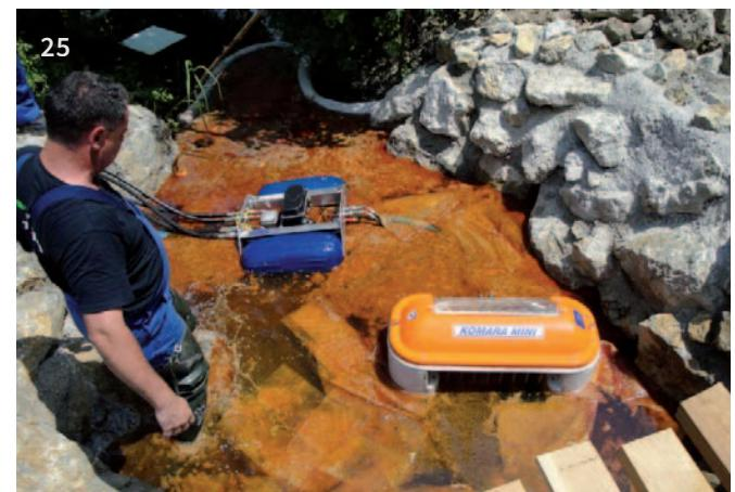
**21** Proper equipment for removing oil products from aquatic areas of rivers, streams, lakes, ponds and the sea
